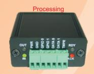
Converter enter in processing mode when receive: - A Wiegand frame - A Command from serial interface
